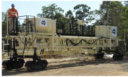
The TC1500 is available with four tracks which offers the best possible weight distribution and lowest ground pressure even in soft trackline conditions. The optional "flip of the switch" 90 degree steering feature is great for maneuvering/steering around job site, self-loading/steering onto a trailer, crossing bridges, and reducing hand pour sizes.
