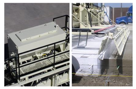
The Cure System is available with a cure tank capacity up to 350 gallons (1,323 L) featuring an oversized access hatch. Cure tank agitation is provided by mechanical agitator and recirculating cure system. As an option, cure hoses can be provided to both sides of the machine to pump cure into the cure tank from barrels or totes. Optional ground level accessible, cure pump on-off switches (located on both sides of the machine) are also available.
