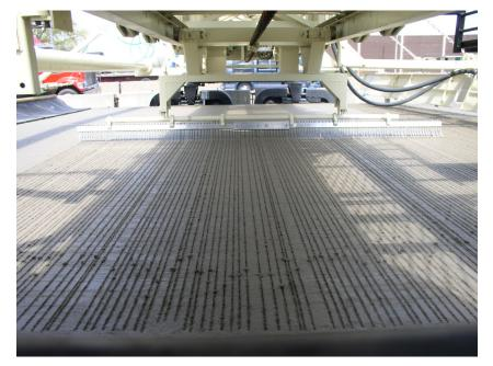
The transverse tining kit uses a hydraulic motor powered chain to drive the tine cart back and forth across the slab in an adjustable track. Movable ramps with limit switches on each end of cart track automatically lift tine rake and stop cart at the end of its travel.
