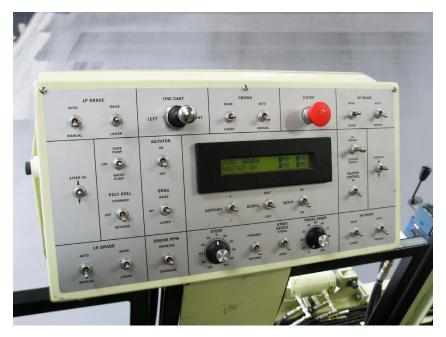
Networked Microprocessor Control System monitors and operates all machine functions including: proportional manual and automatic elevation and steering controls, self-diagnostic capability, counter rotation capability, 90 degree steering mode on four track version, remote engine low idle switch, and constant system monitoring of all sensors.
