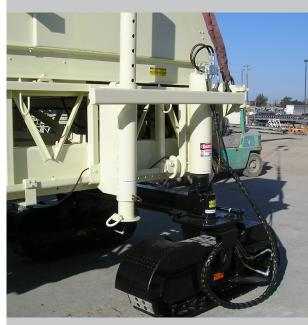
As an option, the TC1500's jacking columns can be equipped with supporting rollers that engage a track system on the main frame. The rollers can be utilized to speed width changes or relocation of the crawler tracks on the track line.
