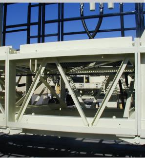
The TC1500's latticework construction is capable of working widths from 12 to 56 ft. (3.65 to 17.06 m). The bottom of the frame sections are pin connected for quick width changes. Each frame section is provided with a hose / cable trough. An optional access walkway with hand railing installed across the entire machine is available.
