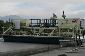
An optional Burlap / Astroturf Drag attachment can be supplied complete with water spray bar. The tow arms can be hydraulically raised/lowered by the operator. Tow arms pivot out of the way for transport. A water system is included with a 60 gallon (227 L) polyurethane tank complete with hydraulic motor driven water pump. As an option, a larger 200 gallon (757 L) polyurethane tank can be supplied.
