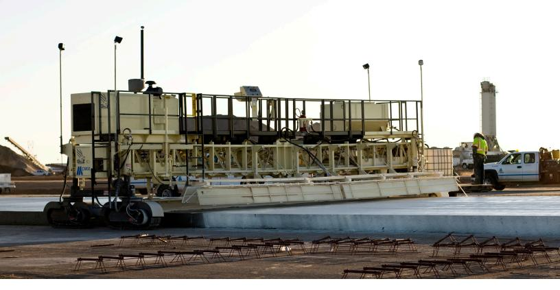
The Guntert & Zimmerman (G&Z) TC1500 is the most technologically advanced texture cure machine on the concrete paving market today. The features contributing to this best-in-class distinction include: 90 degree steering, highly accurate steering and elevation control systems, and unique, rigid frame design for quick width changes.
