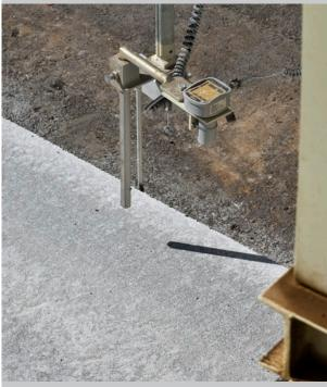
G&Z offers optional ultrasonic sensors and supports for reference off top of slab for elevation control so only one wire is required for steering reference.
