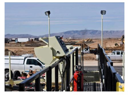
The TC1500 is optionally equipped with an access walkway across the top of the truss frame to optimize operator visibility, speed access, and allow safe movement across the width of the machine. Included in this option, access ladders are provided on each side.
